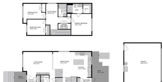
358 WOLF CREEK MANOR SE RECA MEASUREMENT STANDARD - CALGARY 48 Entry Level (AG) - 381.23 Sq Ft / 35.58 m 2 Main Level (AG) - 463.08 Sq Ft / 43.02 m 2 Upper Level (AG) - 824.31 Sq Ft / 76.58 m 2 Total Above Grade RMSD Size - 1648.62 Sq Ft / 153.18 m 2
